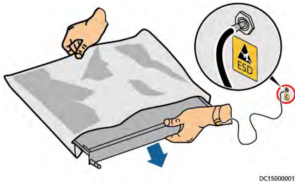
Figure 1-1 Wearing an ESD wrist strap
